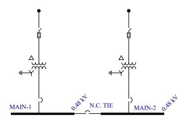
Figure 5.2: Double-End Load Center Configuration
