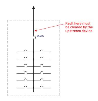
Figure 4.3: Faults on the Line Side of a Main Device
