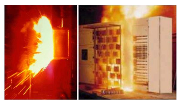
Figure 2.1: (a) Arc Blast in Box; (b) Arcing Fault in an Electrical Panelboard
