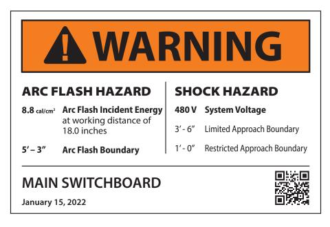
Figure 4.5: Example of an Arc – Flash Warning Label Created by EasyPower
