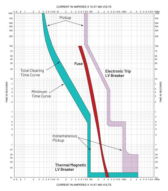
Figure 4.2: Example of TCC Plot with Tolerance Band
