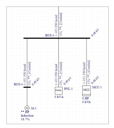
Figure 8.14: Motor, Panel, and MCC are Connected
