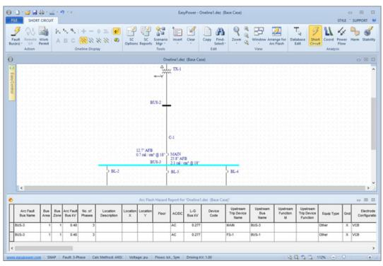
Figure 8.55: Arc Flash Results with the Arc Flash Hazard Report Displayed
