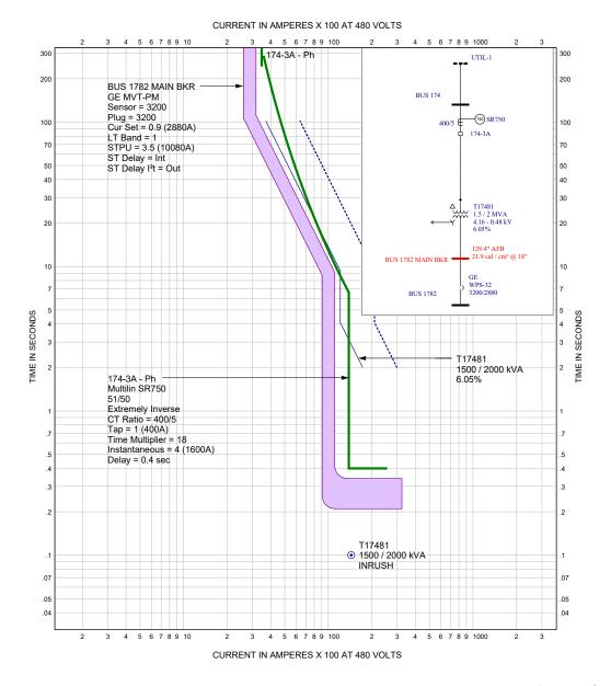
Figure 5.10: Typical Time Overcurrent Curve for a Transformer Primary Relay (Revised)
