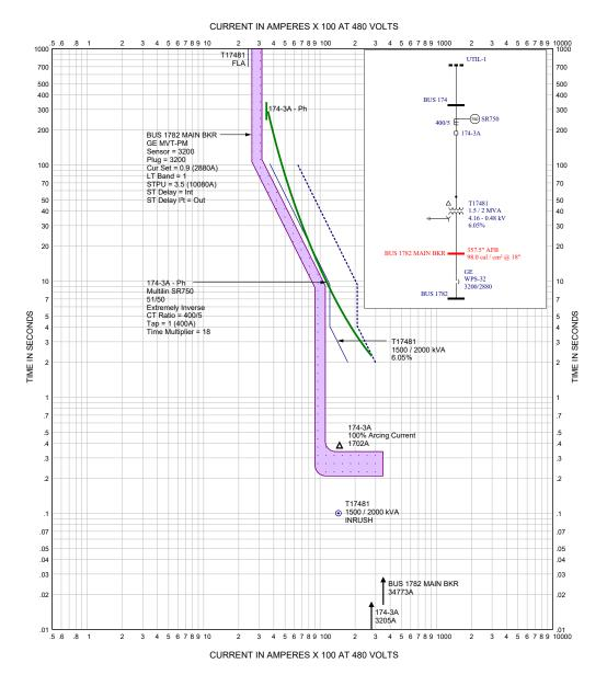
Figure 5.9: Typical Time Overcurrent Curve for a Transformer Primary Relay
