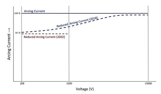
Figure 3.2: Reduced Arcing Current
