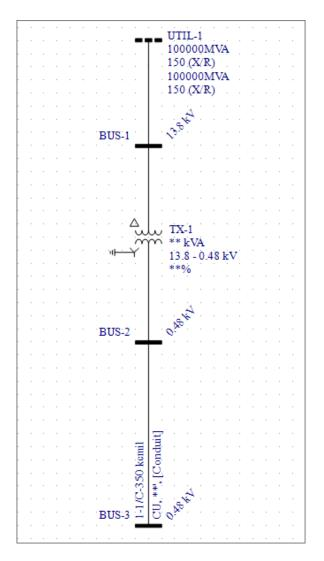
Figure 8.9: Initial One-line Diagram
