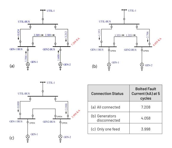
Figure 4.4: Example Showing a Multiple Source Fed Bus Fault and the Series of Operations with the Fault Current Changing with the Breaker Operation
