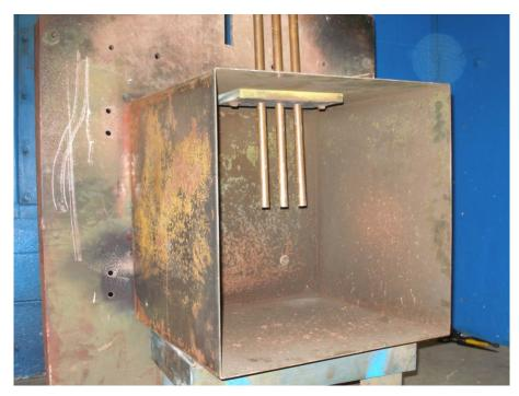
Figure 3.5 – IEEE 1584–2002 Test Setup
