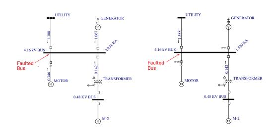
Figure 4.1: EasyPower Example of Connected Equipment for Two Possible Cases
