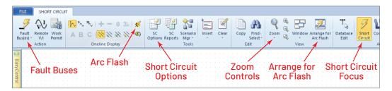
Figure 8.52: Short Circuit Tab Options
