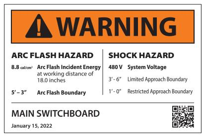
Figure 9.3: ANSI Z535 Arc-Flash Label Example
