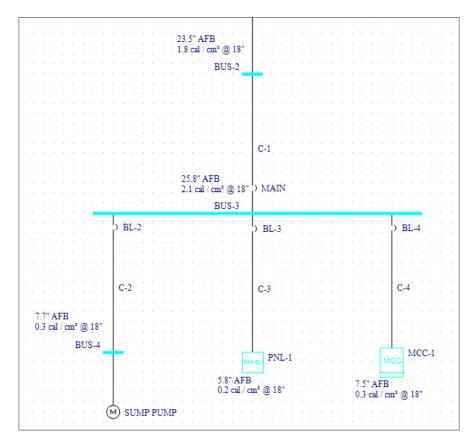
Figure 8.53: Arc Flash Results on the One-line
