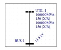
Figure 8.48: Utility Data, Infinite Source
