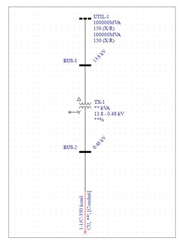
Figure 8.8: Cable Connected to the Transformer
