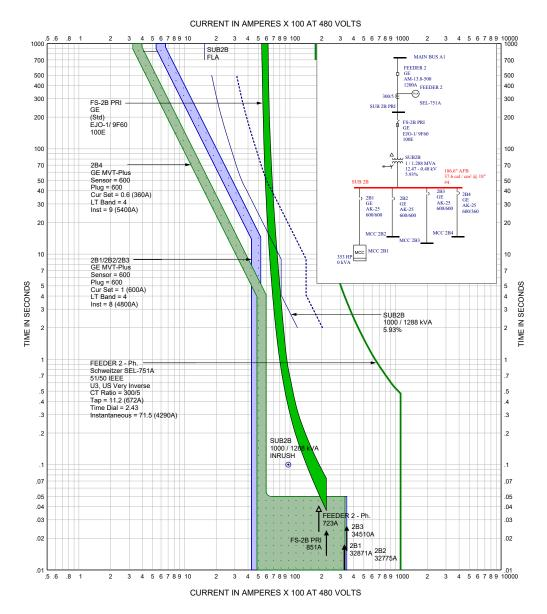
Figure 5.4: Feeder 2 Relay Normal Settings – Arc-Flash at Sub 2B Bus – 37.4 cal/cm<sup>2</sup>
