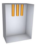
Figure 3.8 – Vertical in Box – No Barrier (VCB)
