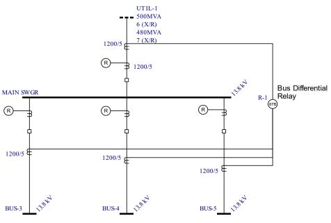
Figure 5.8: Typical Bus Differential Relaying System
