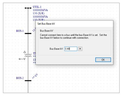
Figure 8.7: Set Bus Base kV on the Secondary Connection
